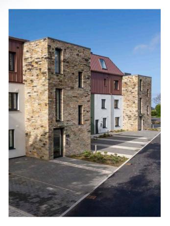
stands out for its use of multiple Fassa systems, tailored to meet the project's high standards. The Fassatherm 'Mechanical Plus' mineral wool system for SFS was chosen for its superior fire protection capabilities, ensuring safety without compromising on aesthetics. Additionally, the project utilised Fassarend render carrier board system '5A'. Allowing for a durable and visually appealing finish. Both systems are certified by Kiwa BDA, underscoring their reliability and quality.
