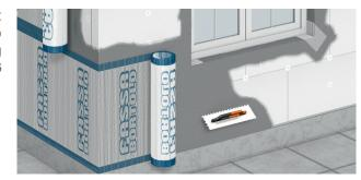
Subsequently, starting from the top down, apply 160 g/m<sup>2</sup> alkali resistant fibreglass reinforcing mesh, with adjacent strips overlapping at least 10 cm, embedded in the base coat A 96; finally, a second base coat is applied so as to obtain a smooth and uniform surface. In addition, two layers of mesh can be used in areas most susceptible to knocks and bumps.
