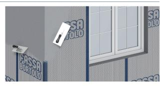
Around five days after application of the base coat, and in any case after the layer of base coat has completely hardened, the primer FX 526, required for the subsequent coloured coating (applied after 16 – 24 hours) is applied by roller or brush. For coloured finish coating use the product RX 561 of the acryl siloxane system. It is not recommended to use dark colours, as in summer this may lead to an excessive increase in surface temperature.
