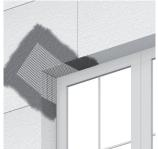
Wait at least two days before applying the base coat, in hot and dry climates, or a maximum of one week in cold and damp climates. The base coat must be applied onto the panels using a metal trowel, apply a uniform thickness of the base coat A 96 of 5-6 mm using a metal trowel.
